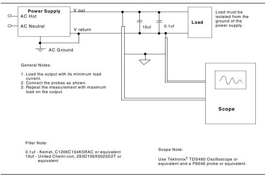
Figure 6. Differential Noise Test Setup
